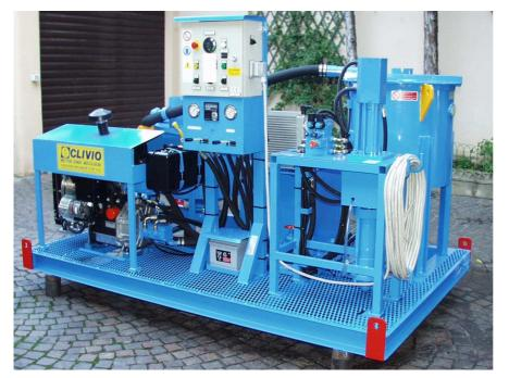
Grout injection unit CLIVIO mod. T.A.D.40-130 DH consisting of:
