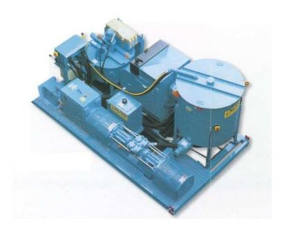
Grout injection unit CLIVIO mod. APOL.SP-DHTA diesel driven consisting of:
