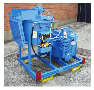
Grout injection unit CLIVIO mod. PS/A-MA140A is air driven and is designed to particularly meet consolidation works in restricted areas where electrical current is not available and where small grouting and low pressure works are required (restauration works, micro piles, foundation, consolidation etc.).
