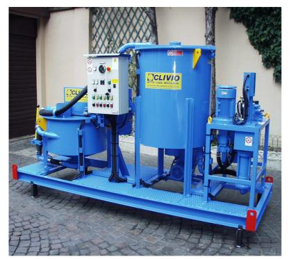
Is designed to meet particularly the problems of consolidation works, micro piling, anchor hole and where valves pipes fracture system is concerned (HP-LP). All machines are properly placed on a single iron welded base for easy operation and prompt site setting.
